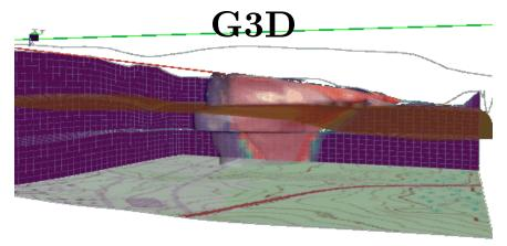
(A Contaminant Plume Infiltrating a Clay Layer)
