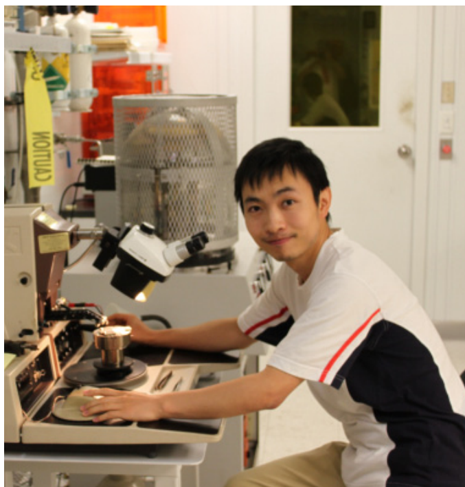
Ning (physics graduate) is using the wire bonding machine to bond gold wire into the sample.
